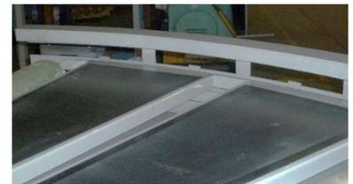
**Tapered End Pulleys:** Supported at each end of the curved frame by 'life greased' ball bearing units fixed to it are tapered conical pulleys manufactured in high density polypropylene on a steel shaft. These two pulleys can be adjusted in the horizontal plane by tensioning devices to provide the correct amount of tension in the belt. Each pulley is removable independently from the side of the belt bend.
