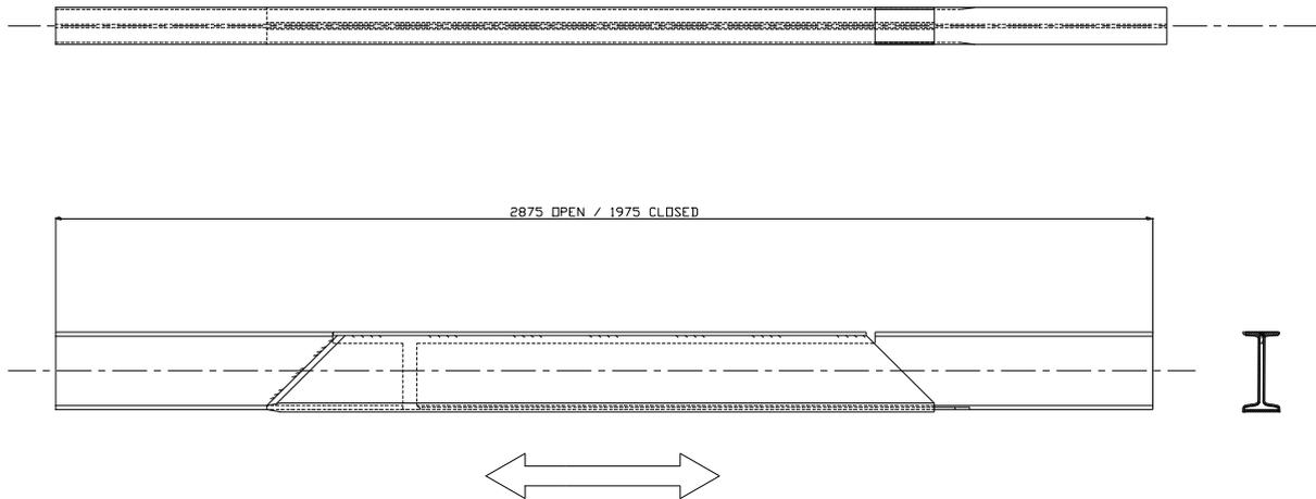
The construction of the unit is similar to that of a linear tension unit, with the use of a track section sliding within a 'sleeved section'.
