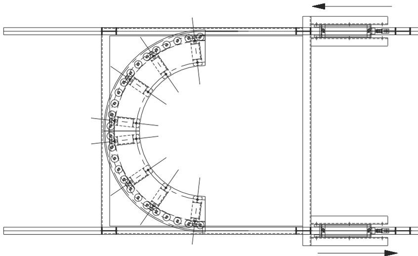
This framework allows chain tensioning to be carried out without the necessity to adjust any conveyor supports.
