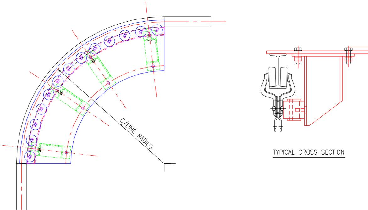
The hardened roller turn rollers are used to resist the turning moment of the conveyor chain and retain it in the centre line, due to the working chainpull.
