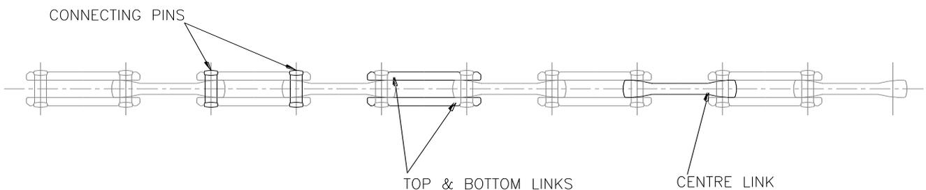
Once this assembly is tensioned the chain section is formed.
