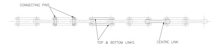
Once this assembly is tensioned the chain section is formed.
