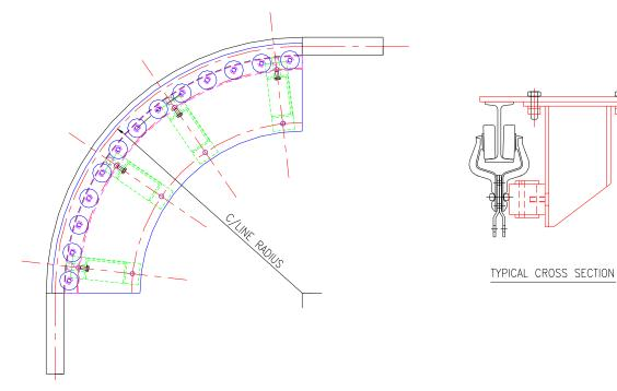
The hardened roller turn rollers are used to resist the turning moment of the conveyor chain and retain it in the centre line, due to the working chainpull.
