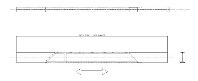
The construction of the unit is similar to that of a linear tension unit, with the use of a track section sliding within a 'sleeved section'.
